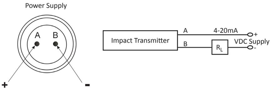
**Figure 2:** Basic connection diagram for normal operation
